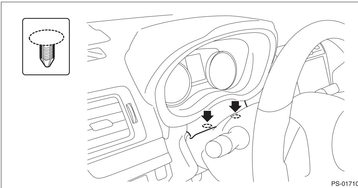
(2) Remove the screws by turning the steering wheel to right and left.
